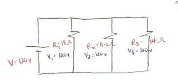
\* in a parallel circuit, all resistors have the same voltage.
